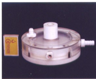
Fig. 7. Photo and diagram of the cell of the water electric generator of heat (patent No. 2258098)
