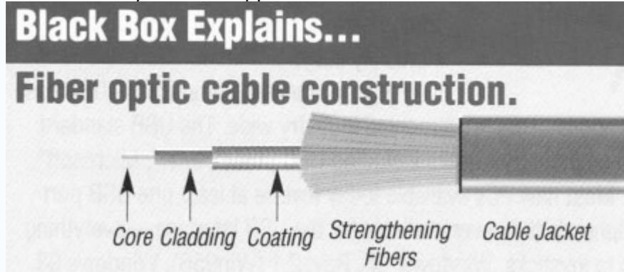
**The operating principle of optical fibers** applies to a number of variants including single-mode optical fibers, graded-index optical fiber, and step-index optical fibers. Because of the physics of the optical fiber, special methods of splicing fibers and of connecting them to other equipment are needed. A variety of methods are used to manufacture optical fibers, and the fibers are also built into different kinds of cables depending on how they will be used.
