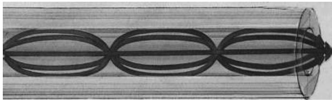
reducing its travel distance. The shortened path and the higher speed allow light at the periphery to arrive at a receiver at about the same time as the slow but straight rays in the core axis. The result: a digital pulse suffers less dispersion.
