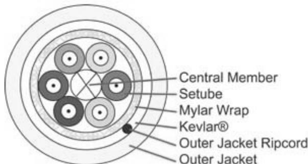
insulates fibers from stresses of installation and environmental loading. Buffer tubes are stranded around a dielectric or steel central member, which serves as an anti-buckling element.
