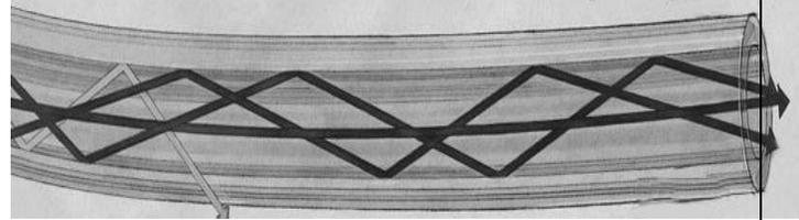
**GRADED-INDEX MULTIMODE FIBER** contains a core in which the refractive index diminishes gradually from the center axis out toward the cladding. The higher refractive index at the center makes the light rays moving down the axis advance more slowly than those near the cladding. Also, rather than zigzagging off the cladding, light in the core curves helically because of the graded index,
